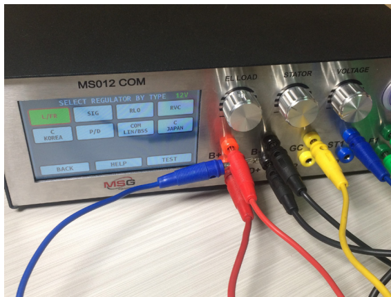
Figure 19 – Connection of additional cable B+
