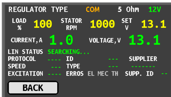
Figure 12 – Diagnostic screen for 12V voltage regulators of COM type
